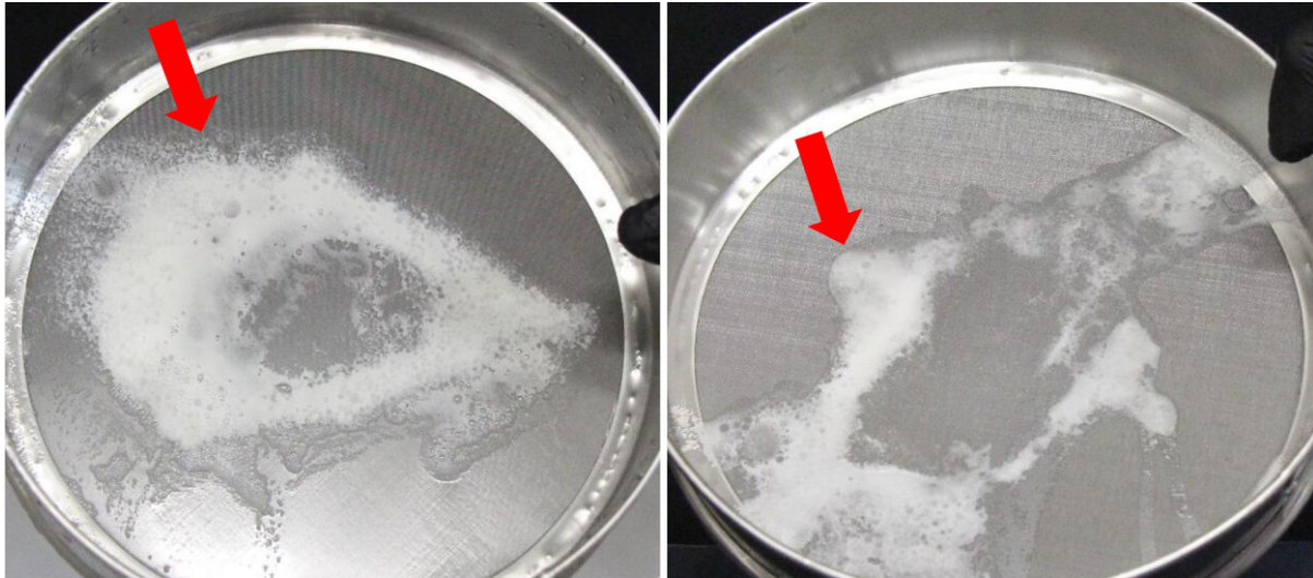
Example of compatibility problem of mixtures with gli wg1 + 2,4-D at application rates of 40 L/ha (a) and 80 L/ha (b) with residues, similar to foam, on 100 mesh sieves
