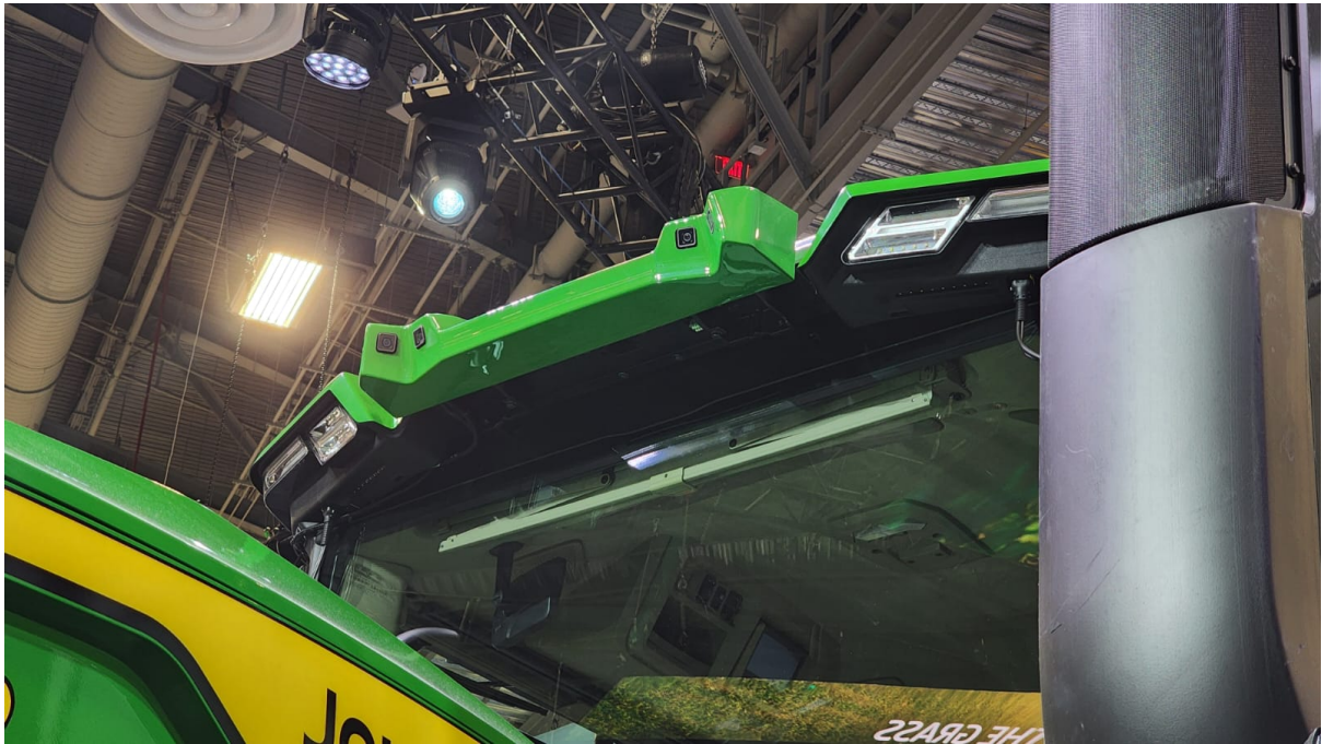
Cameras on the autonomous 9RX tractor
