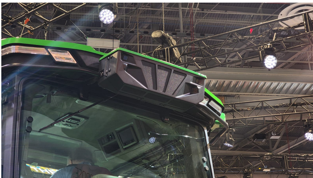
Cameras on the autonomous 9RX tractor
