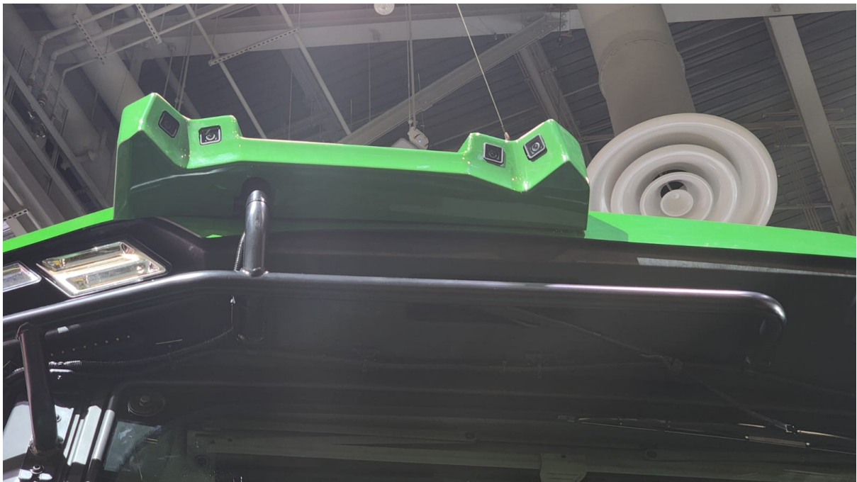
Cameras on the autonomous 9RX tractor
